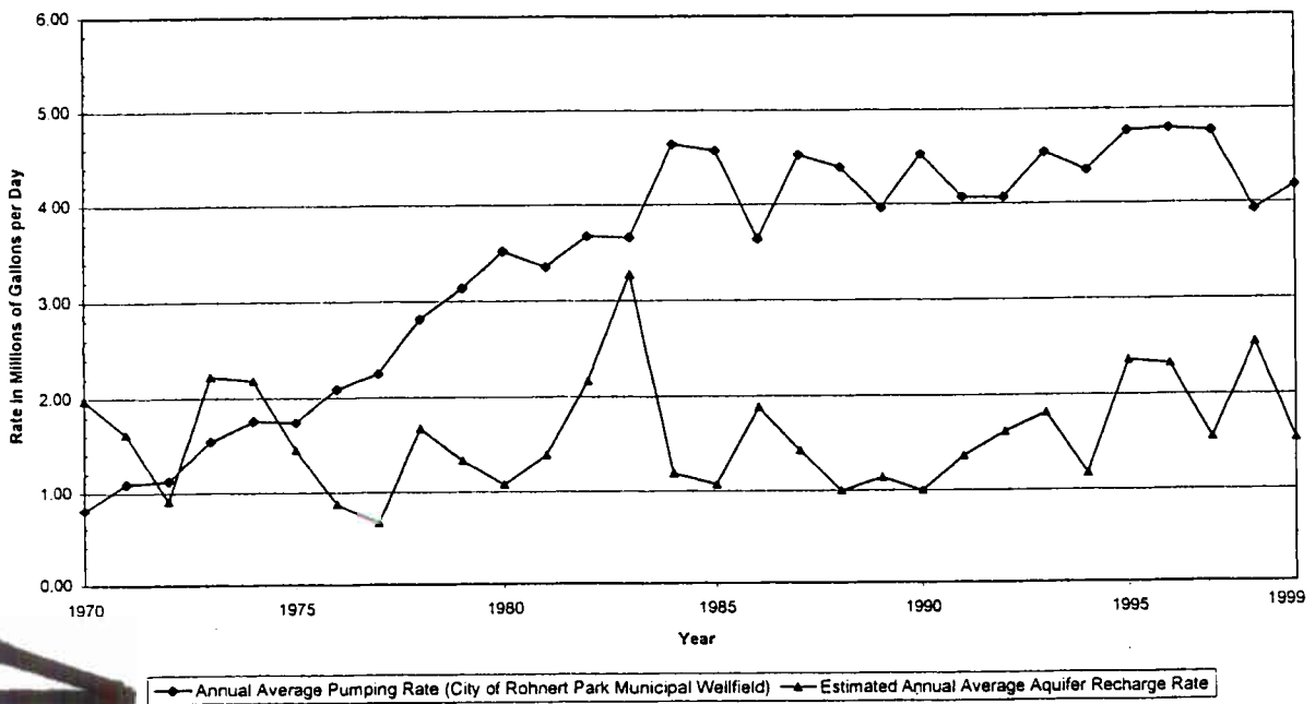
Figure 4.10-2. Annual Average Rates of Recharge and Pumping MODFLOW Groundwater Simulations 1970 through 1999
