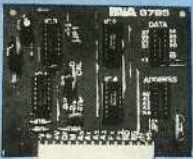
8785 LINEAR DIGITAL TO ANALOG CONVERTER RETRO-FITS EXPONENTIAL SYNTHESIZERS TO PAIA DIGITAL (see page 9)
