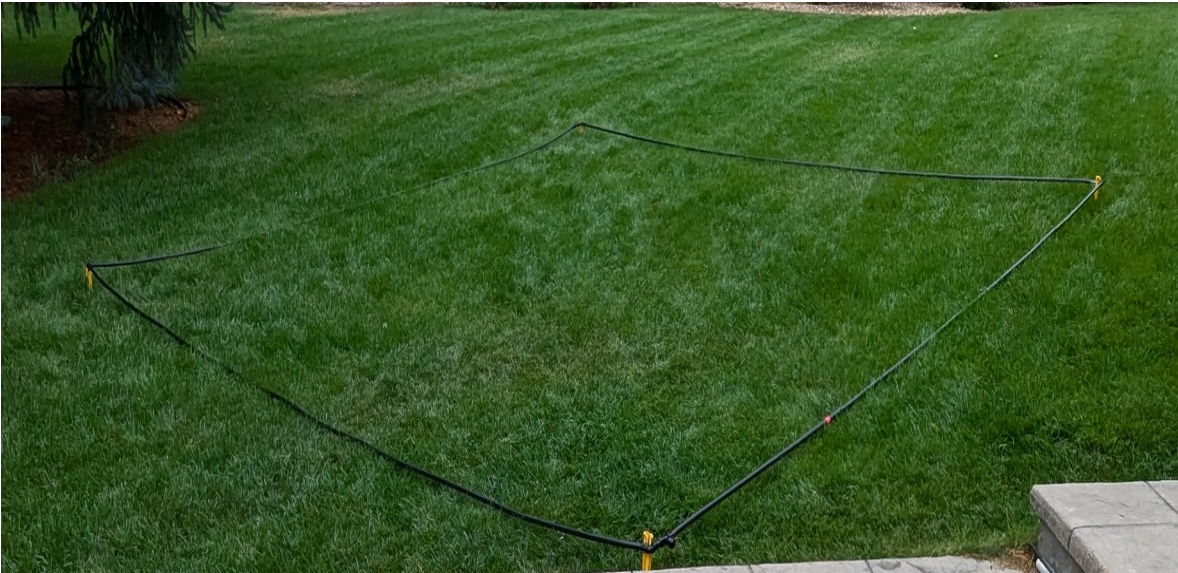
Figure 6: 5m/side square LoE #25AWG conductor enclosed in .5" drip water line 10-20cm above the earth
