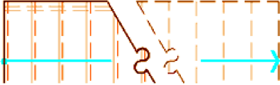
STAIR LINE - STRAIGHT, ENTIRE STAIR ARROW = CUSTOM DIM STYLE BREAK MARK = CURVED
